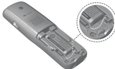
2. Align the cover flat against the battery compartment, then slide it upwards until it clicks into place.
